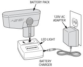
When fully charged, reattach battery pack onto Cordless Jigsaw, making certain latches fasten securely. Cordless Jigsaw will not operate properly if the battery pack is not seated properly.
